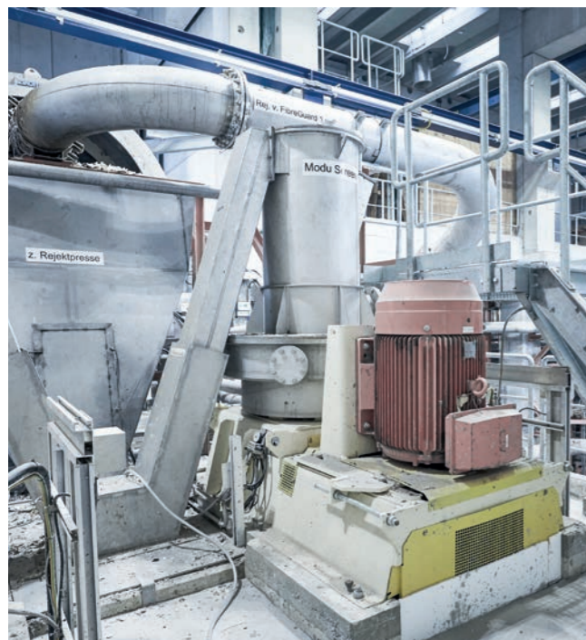
ModuScreens TD tailing screens are part of coarse screening. Efficient washing of fibers is done with a FibreWash Drum – one important part of the detashing system.
