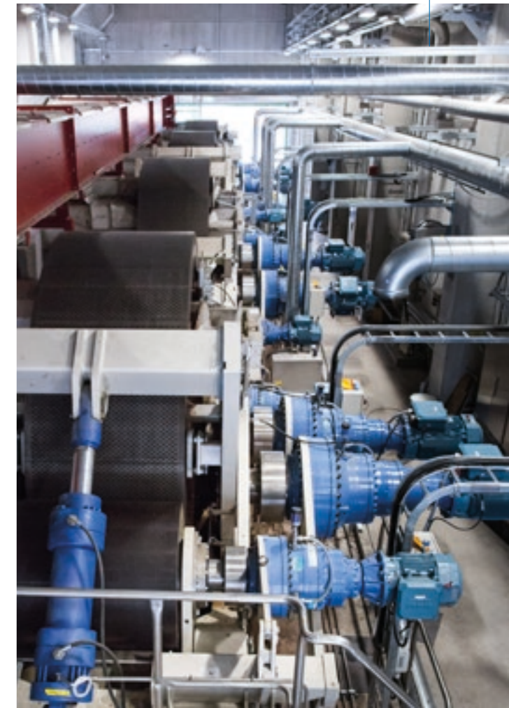
One of the new, key technologies introduced to the woodyard is the new generation bark press, ANDRITZ HQ-Press, which targets to deliver around 5%-unit higher dry solids content of bark than any other press on the market.
