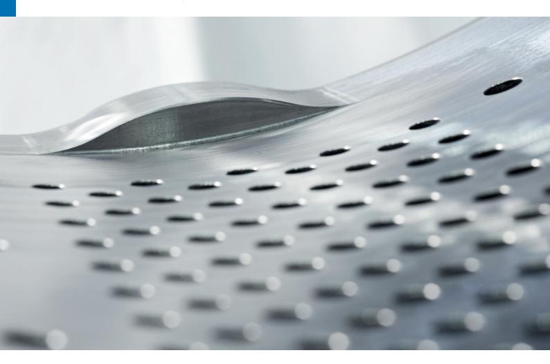
The ANDRITZ Eco Repair concept reduces repair costs drastically and eliminates technical disadvantages. As welding is no longer needed, the original geometry of the compres-
